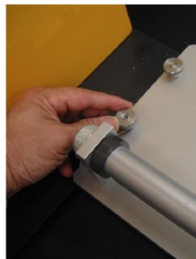
Figure 7 - Spin thread onto bobbin
