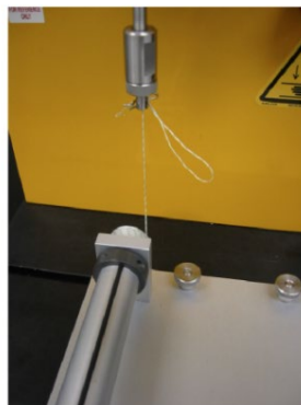
Figure 8 - Raise the arm & remove any slack
