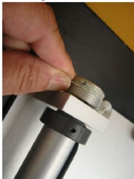
Figure 6 - Secure fixture to CTX base
